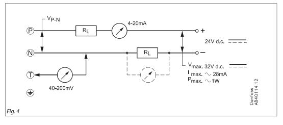
The transmitter has a wiring diagram, see fig. 4. Terminals P (positive) and N (negative) are connection terminals for the supply voltage. The same leads are used for supply voltage and output signal. A function test can be performed between terminals N and T without cutting off the current loop.
