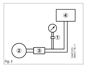
In cases where valves are closed momentarily, surges of a value in excess of that for which the pressure element is designed can occur. To avoid damage to the pressure element, a damper should be fitted.
