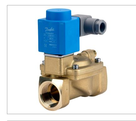
EV224B for compressed air, is a high pressure indirect servo-operated 2/2-way solenoid valve with working pressure up to 40 bar, medium temperature up to 60 °C and available in NC and NO versions.
