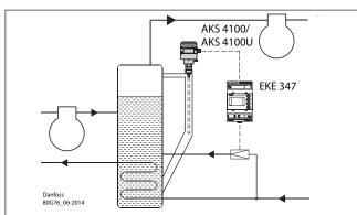
System configuration AKV/A Regulating principle: Low Level Signal setup: AKS 4100/U
