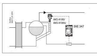
System configuration AKV/A Regulating principle: Low Level Signal setup: AKS 4100/U
