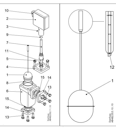
AKS 38 incorporates an internal float assembly (1), which will operate directly in accordance with the refrigerant level.
