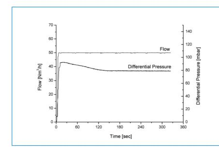
Dewetting characteristic of a P-SRF N 05/25 after steaming at 1 bar for 30 minutes. Flow is 50 Nm<sup>3</sup>/h at 1,2 bar absolute. Normal conditions are reached after ~ 150 seconds.
